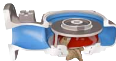
Stage 1. Most solids entering the pump pass through the impeller between the impeller vanes. If a solid object gets caught on the leading edge of one of the vanes, it slides along the backswept shape towards the perimeter of the inlet.
